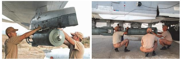
The two above photos show technicians attaching FAB 250 bombs to the undercarriage of an aircraft. This variant of the munition could be a high explosive bomb weighing about 250 kg (about 550 pounds) or possibly a bomb that carries submunitions that are dispersed over a target. The standard munition is simply the equivalent of the 500 pound bomb used by the United States Air Force.
